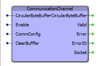
The functions in this user library make it easy to incorporate advanced controller communications such as email and FTP. Also included is a set of function blocks to simplify the creation of a custom ASCII command / response interface with other equipment using and Ethernet or serial connection.
